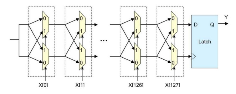
(picture from Heder et al.: Physical unclonable Functions and applications)
